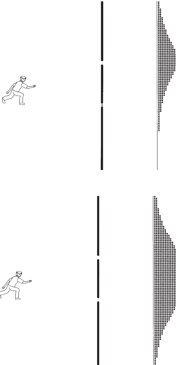
FIGURE 2-1 Blindfolded bowler with one gate open (top) and two gates open (bottom). Balls that hit the fence are assumed to be removed; the pattern shown is the average that would result if the experiment was repeated a large number of times.
